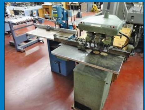
Three-Spindle and Single-Spindle Paper Drills
